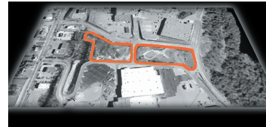
Typical out parcels that should be linked to internal circulation roads only
